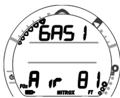
Fig. 89 - GAS 1 SWITCH PREVIEW
