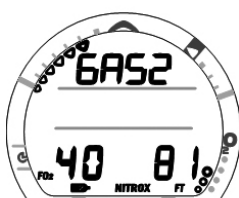
Fig. 90 - GAS 2 SWITCH PREVIEW
