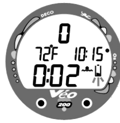
Fig. 9 -Low Battery Condition
