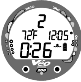
Fig. 68 - Surface Mode (greater than 10 minutes)
