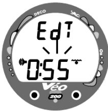
Fig. 22 - Set Elapsed Dive Time Alarm
