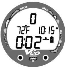
Fig. 16A- Surface Mode (module is dry)
