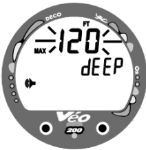
Fig. 21 - Set Max Depth Alarm
