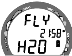
Fig. 76 - Fly Mode (Activation Contacts Wet)
