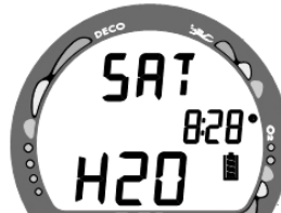
Fig. 77 - Desaturation Mode (Activation Contacts Wet)
