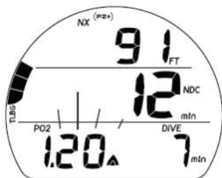
Fig. 72 - PO2 WARNING (during audible)
