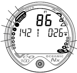
Fig. 45 - VIOLATION GAUGE MODE
