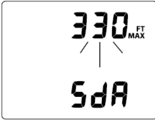
Fig. 24 - SET DEPTH ALARM
